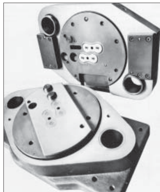
A fine-blanking tool made from Sverker 3, for the manufacture of chain links for precision roller chains.
