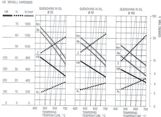
Hardening at 830-850°C with quenching in oil. Soaking time in minutes when the surface has attained full temperature, is 0.7 x thickness in mm. Interrupt the quenching at 125°C and temper immediately afterwards.
